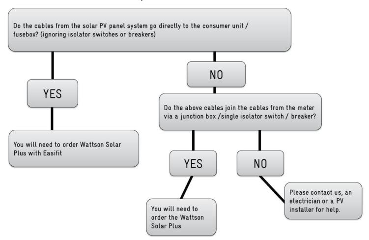
Wattson Classic doesn't require an Easifit and can usually be installed by the end-user. This is because in the vast majority of homes, the single-core cables that the sensor fits around are easy to access coming out of the meter or going into the fuse board.
